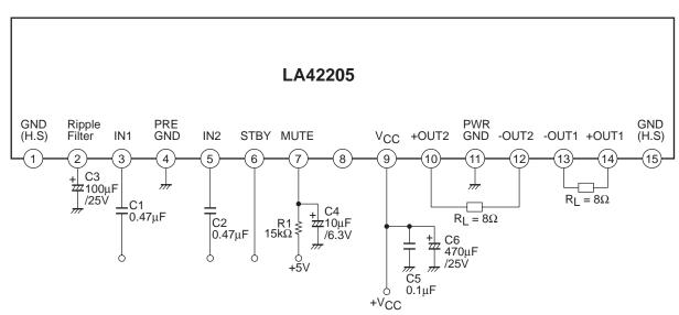
\* Pin 8 : NC. This pin must be left open.
