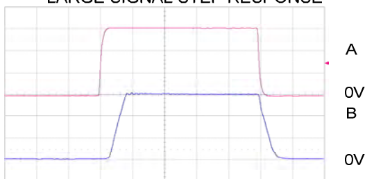
OPERATIONAL - AMPLIFIER LARGE SIGNAL STEP RESPONSE
